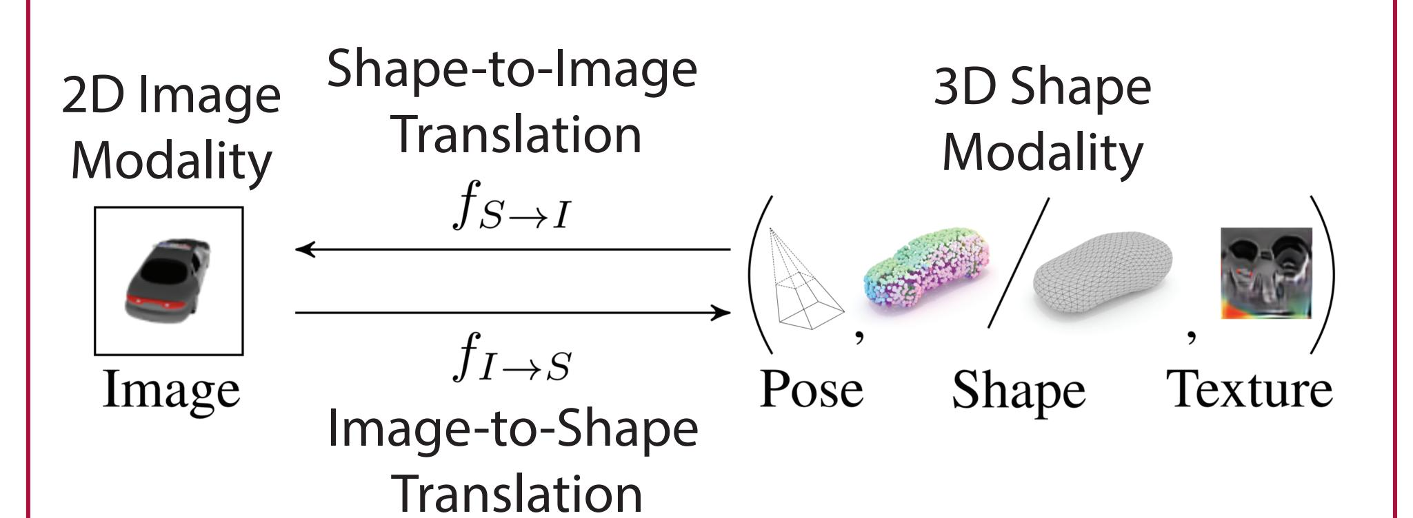
Our 3D shape representation is a **graphics code**, consisting of a rigid pose, a deformable mesh, and a 3D texture.
